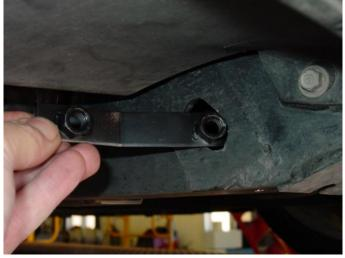
7.) While holding the nut plate in place, locate the rear tow hook into position so that the slots in the tow bracket line up with the holes in the frame rail and the nut plate and insert the screws with washers and finger tighten the screws.
