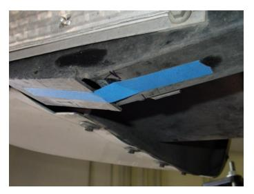
3.) Draw a line down the center of the frame, and then draw a line across the frame 1" from the frame line on the bottom. Now draw a line across the upper frame rail 2 <sup>1</sup>/<sub>4</sub>" from the frame line.
