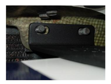
3.) After positioning the tow bracket to allow clearance around it, tighten the hex nuts securely.
